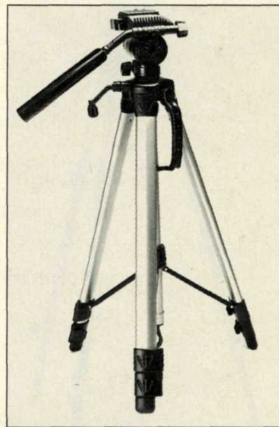
▲ Above: This is an example of a lightweight tripod with three way-pan head and leg braces. Other features of the Vivitar VPT-120 Video/Photo tripod are a crank-operated center column, a removable quick-release camera platform and a built-in circular bubble level. The unit is fitted with a carrying handle.
